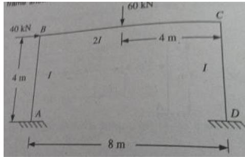
5. Analyse the frame as shown in figure below by moment distribution method. 10M
