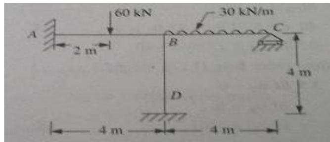
3. Analyse a frame shown in figure below by Slope deflection method. 10M
