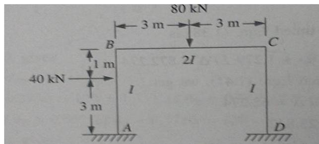
4. Analyse a frame shown in figure below by Slope deflection method. 10M
